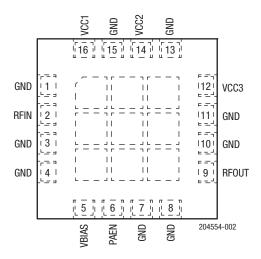
Figure 2. SKY66391-12 Pinout (Top View)
