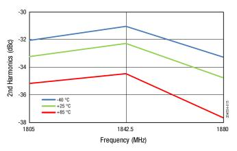
Figure 11. Second Harmonic @ +28 dBm (CW) vs Frequency Across Temperature
