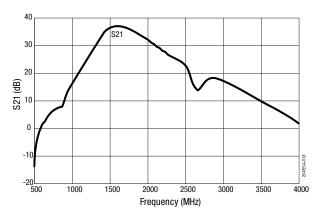
Figure 14. Wide Band Small Signal Gain vs Frequency
