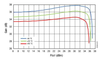
Figure 7. Gain vs. Pout Across Frequency
