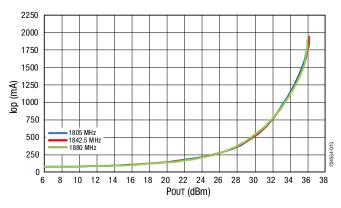
Figure 9. Iop vs. Pout Across Frequency
