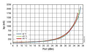
Figure 10. lop vs Pout Across Temperature
