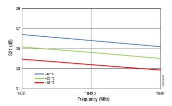
Figure 13. S21 vs Frequency Across Temperature (Pin = -20 dBm)
