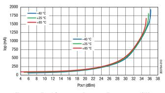
Figure 10. Total Current vs. Pout over Temperature (CW)
