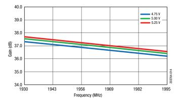
Figure 14. Gain @ Pout = +28 dBm vs Frequency over Voltage
