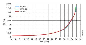
Figure 9. Total Current vs. Pout over Frequency (CW)
