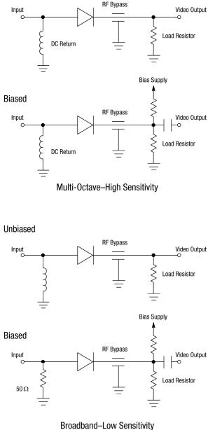
**Figure 5. Typical Video Detector Circuits**
