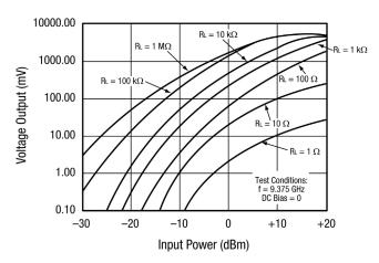
Figure 3. Voltage Output vs Input Power as a Function of Load Resistance
