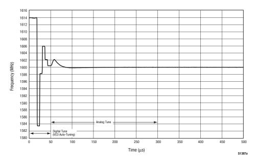
Figure 7. VCO Auto-Tuning @ 1600 MHz Frequency Settling
