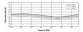
Figure 27. Phase Noise @ 6 MHz Offset vs Frequency and Supply Voltage
