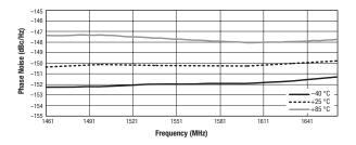
Figure 24. Phase Noise @ 1.8 MHz Offset vs Frequency Temperature
