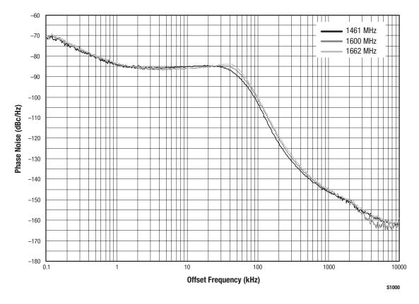
Figure 8. SKY73103-11 Single Sideband Phase Noise Measurements
