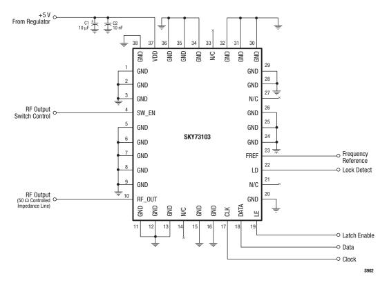
Figure 28. SKY73103-11 Typical Application Schematic
