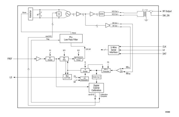
Figure 2. SKY73103-11 Functional Block Diagram
