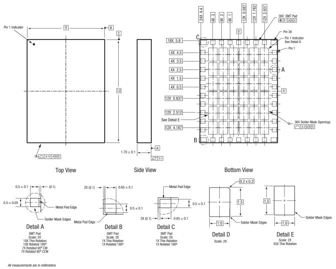
Dimensioning and tolerancing according to ASME Y14.5M-1994.
