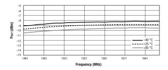
Figure 10. Output Power vs Frequency and Temperature
