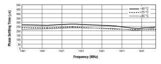
Figure 14. Phase Settling Time vs Frequency and Temperature
