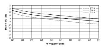
Figure 13. Mixer A IIP3 vs Frequency and Supply Voltage
