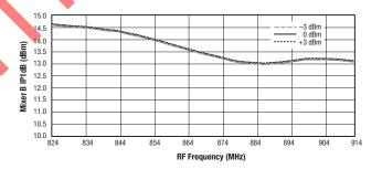
Figure 24. Mixer B Input P1dB vs Frequency and L0 Power
