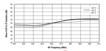
Figure 28. Mixer B RF to IF Isolation vs Frequency and Temperature
