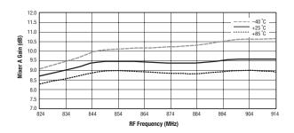
Figure 4. Mixer A Gain vs Frequency and Temperature
