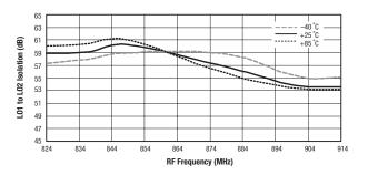
Figure 32. L01 to L02 Isolation vs Frequency and Supply Voltage
