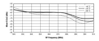
Figure 26. Mixer B 2RF-2LO vs Frequency and Temperature
