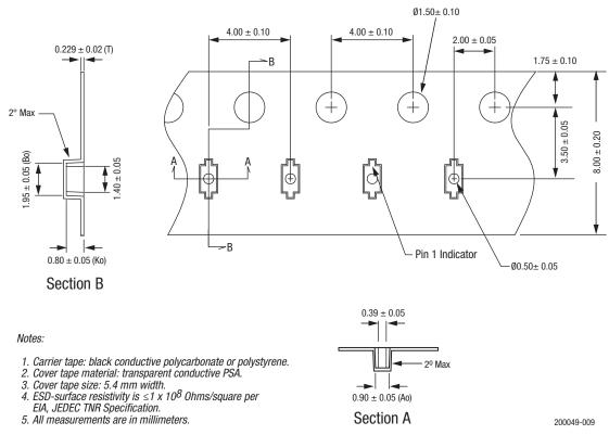
Figure 8. SC-79 Tape and Reel Dimensions
