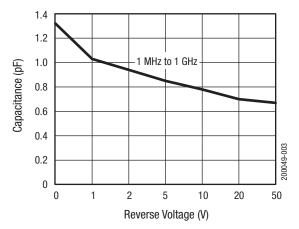
Figure 3. Capacitance vs Reverse Voltage
