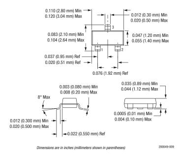
Figure 9. SOT-23 Package Dimension Drawing
