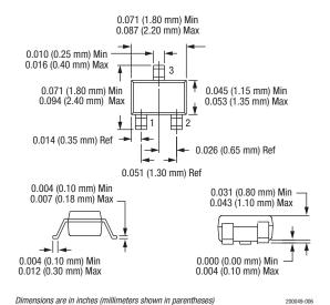
Figure 5. SC-70 Package Dimension Drawing
