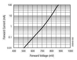
Figure 2. Forward Current vs Voltage
