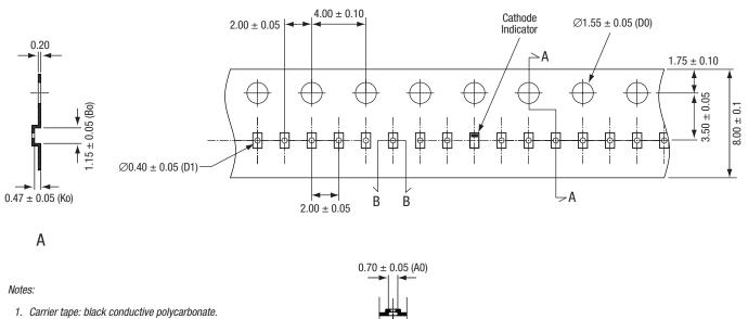
Cover tape: transparent conductive polycarbonate Cover tape: transparent conductive material. Cover tape size: 5.4 mm width. 2. 3.
