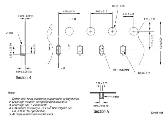
Figure 8. SC-79 Tape and Reel Dimensions
