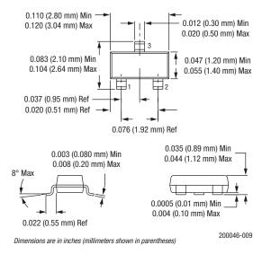
Figure 9. SOT-23 Package Dimension Drawing
