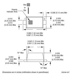
Figure 7. SC-79 Package Dimension Drawing
