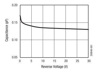
Figure 1. Total Capacitance vs Reverse Voltage
