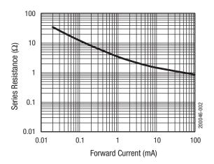
Figure 2. Series Resistance vs Current @ 100 MHz
