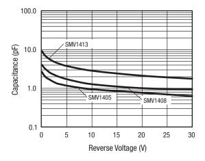
Figure 1. Capacitance vs Reverse Voltage
