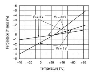
Figure 2. Relative Capacitance Change vs Temperature
