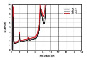
Figure 14. K Stability vs Frequency Over Temperature
