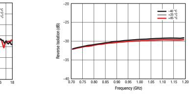
Figure 8. Narrowband Reverse Isolation vs Frequency Over Temperature
