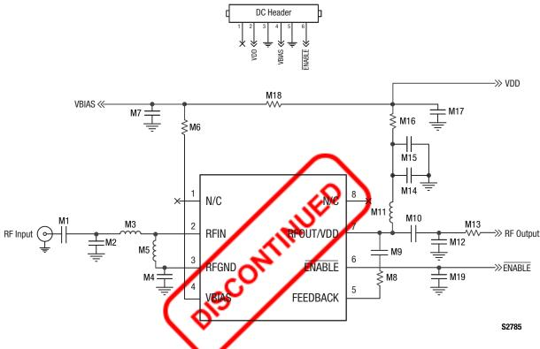
Figure 25. SKY67111-396LF Evaluation Board Schematic
