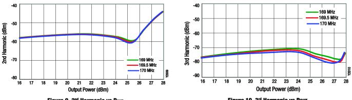
Figure 9. 2<sup>nd</sup> Harmonic vs Pout
