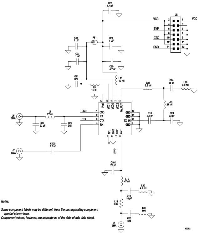
Figure 13. SKY66100-11 EK-2 Evaluation Board Schematic (+27 dBm)
