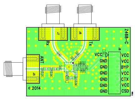
Figure 14. SKY66100-11 Evaluation Board Assembly Drawing (Applies to both EK-1 and EK-2 Evaluation Boards)
