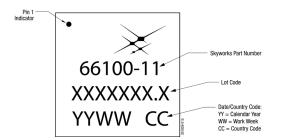
Figure 15. Typical Part Marking
