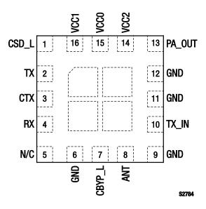
Figure 2. SKY66100-11 Pinout - 16-Pin MCM (Top View)
