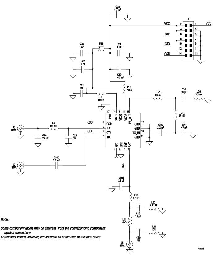
Figure 12. SKY66100-11 EK-1 Evaluation Board Schematic (+24 dBm)
