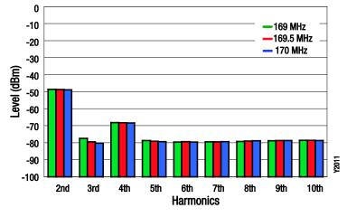
Figure 11. Harmonics at POUT = +27 dBm
