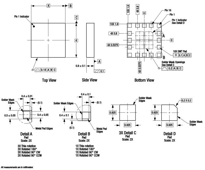
Dimensioning and tolerancing according to ASME Y14.5M-1994
