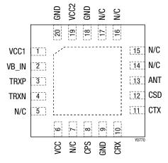
Figure 2. SKY66108-11 Pinout—20-Pin QFN (Top View)
