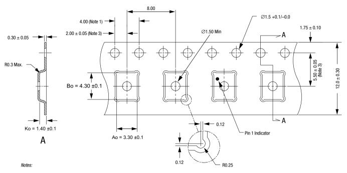
10 sprocket hole pitch cumulative tolerance  $\pm 0.2$  mm. Camber in compliance with EIA 481.
