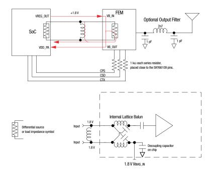
The balun at the FEM PA input (or LNA output) can also be used to inject a bias operating point for the transceiver output stage (the shunt inductor provides a DC path on the other side). The inductor also tunes out any parasitic capacitance.
