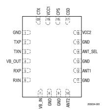
Figure 1. SKY66109-11 Pinout (Top View)
