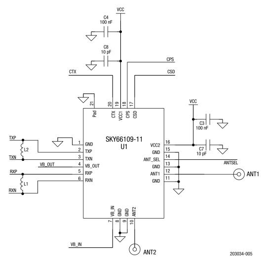
Figure 5. SKY66109-11 Reference Design Schematic
