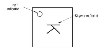
Figure 13. Typical Part Markings (Top View)
