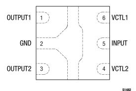
Figure 2. SKYA21012 Pinout (Top View)
