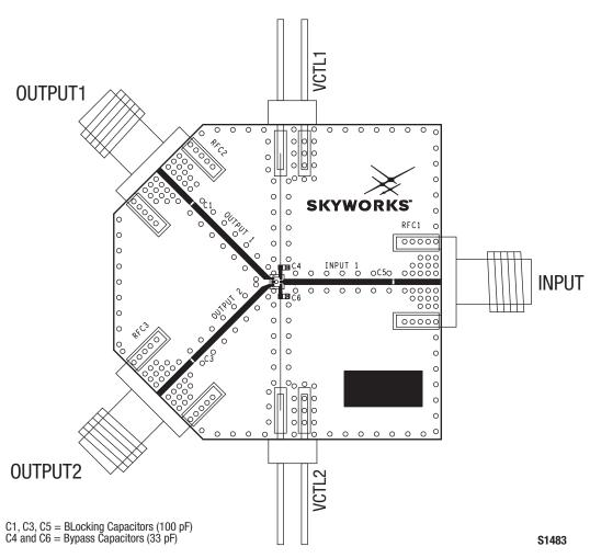
Figure 11. SKYA21012 Evaluation Board Assembly Diagram
