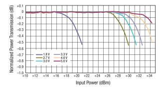
Figure 7. Compression vs Control Voltage (5.2 to 5.8 GHz)
