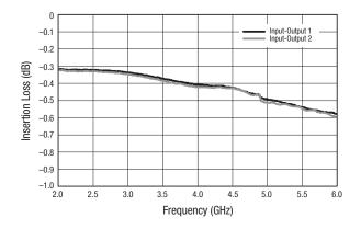
**Figure 3. Typical Insertion Loss**
