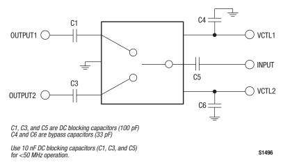
Figure 10. SKYA21012 Evaluation Board Schematic
