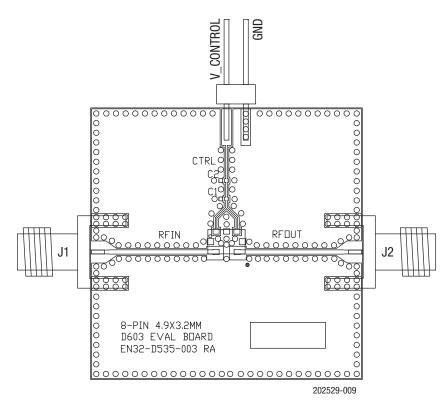
Figure 9. SKY12236-11 Evaluation Board Assembly Diagram
