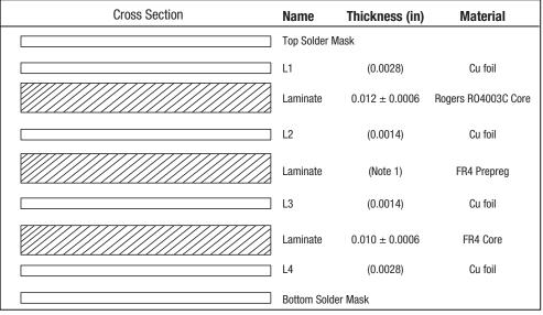
Note: Adjust this thickness to meet total thickness goal of  $0.062 \pm 0.005$  inches.
