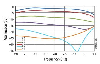
**Figure 3. Attenuation vs Frequency Over Control Voltage**
