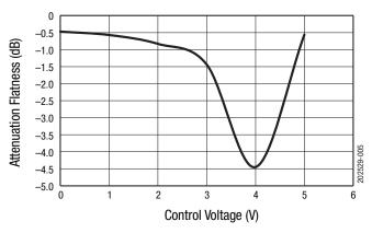
Figure 5. Attenuation Flatness vs Control Voltage (f = 3.3 to 4.3 GHz)
