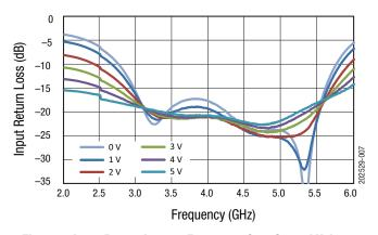
Figure 7. Input Return Loss vs Frequency Over Control Voltage
