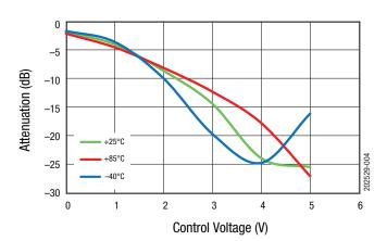
Figure 4. Attenuation vs Control Voltage Over Temperature (f = 3.8 GHz)
