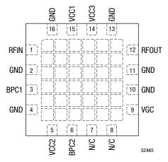
Figure 2. SKY65372-11 Pinout (Top View)
