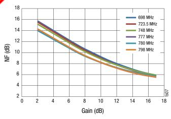
Figure 6. NF vs Low Gain over Different Frequency
