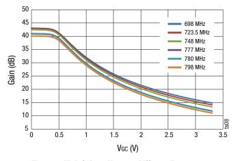
Figure 7. High Gain vs Vgc over Different Frequency
