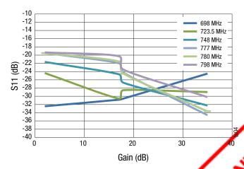
Figure 3. S11 vs Gain over Different Frequency
