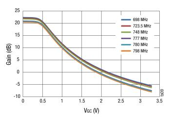
Figure 8. Low Gain vs Vgc over Different Frequency
