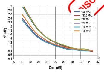
Figure 5. NF vs High Gain over Different Frequency
