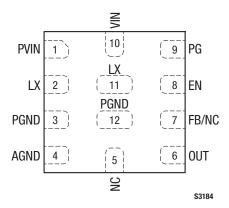
Figure 2. SKY87202-11/-12 Pinout – 12-Pin QFN Packages (Top View)
