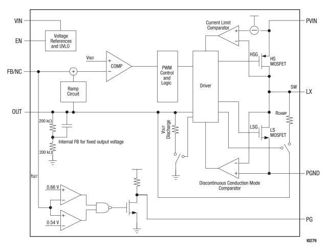
Figure 3. SKY87202 Functional Block Diagram
