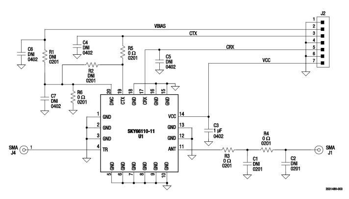
Figure 3. SKY66110-11 Evaluation Board Schematic
