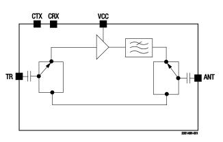
Figure 1. SKY66110-11 Functional Block Diagram
