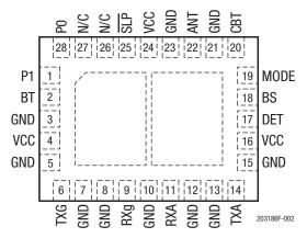
Figure 2. SKY85806-11 Pinout (Top View)
