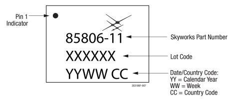
Figure 7. SKY85806-11 Typical Part Markings (Top View)
