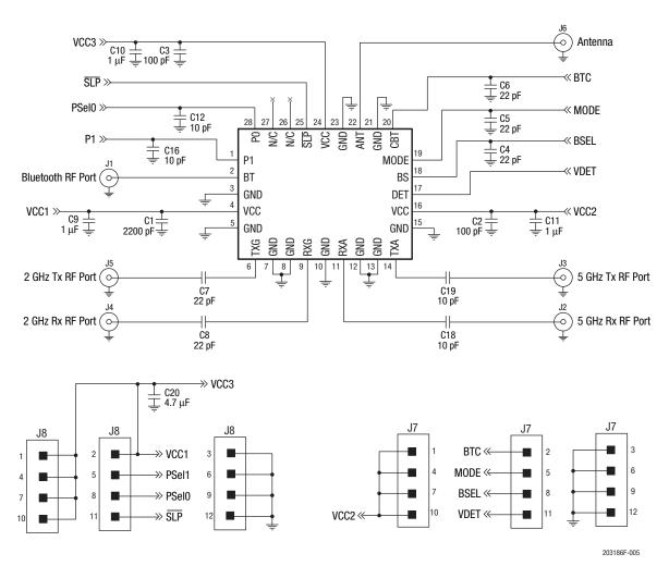
Figure 5. SKY85806-11Evaluation Board Schematic
