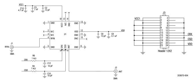
Figure 4. SKY66113-11 Evaluation Board Schematic Diagram
