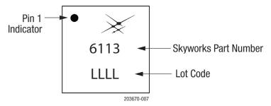
Figure 7. SKY66113-11 Typical Part Marking (Top View)
