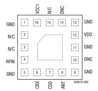
Figure 2. SKY66113-11 Pinout (Top View)
