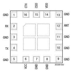
Figure 2. SKY66115-11 Pinout (Top View)
