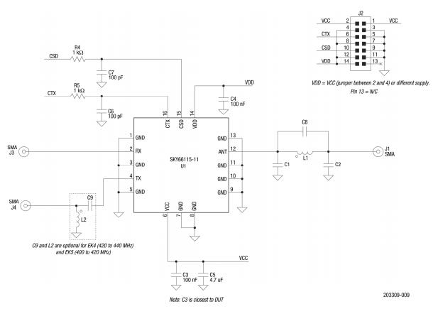
Figure 9. SKY66115-11 Evaluation Board Schematic
