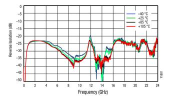
Figure 21. Broadband Reverse Isolation vs Frequency over Temperature
