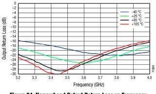
Figure 24. Narrowband Output Return Loss vs Frequency over Temperature
