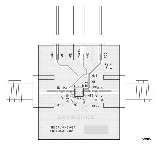
Figure 36. SKY67159-396LF Evaluation Board Assembly Diagram
