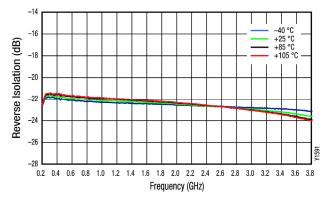
Figure 8. Narrowband Reverse Isolation vs Frequency over Temperature
