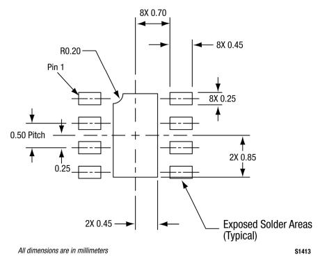
Figure 40. SKY67159-396LF PCB Layout Footprint (Top View)
