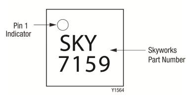
Figure 41. Typical Part Markings (Top View)
