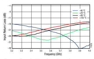
Figure 18. Narrowband Input Return Loss vs Frequency over Temperature
