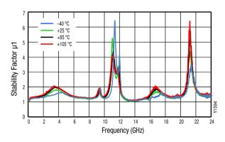
Figure 12. Stability Factor ( $\mu$ 1) vs Frequency over Temperature
