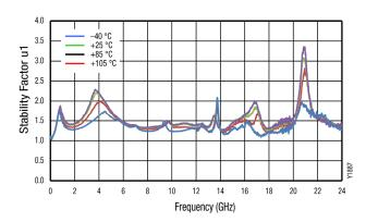
Figure 26. Stability Factor u1 vs Frequency
