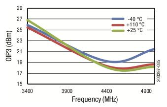
Figure 35. OIP3 vs Frequency over Temperature
