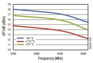
Figure 34. OP1dB vs Frequency over Temperature
