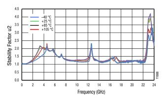
Figure 27. Stability Factor u2 vs Frequency
