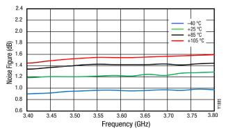
Figure 25. Noise Figure vs Frequency
