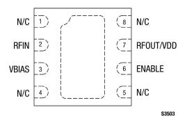
Figure 2. SKY67159-396LF Pinout (Top View)
