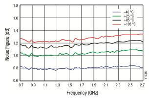
Figure 3. Evaluation Board NF vs Frequency over Temperature
