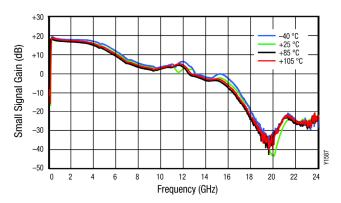
Figure 5. Broadband Gain vs Frequency over Temperature
