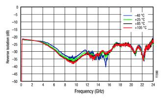
Figure 9. Broadband Reverse Isolation vs Frequency over Temperature
