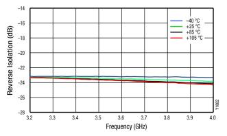
Figure 22. Narrowband Reverse Isolation vs Frequency over Temperature
