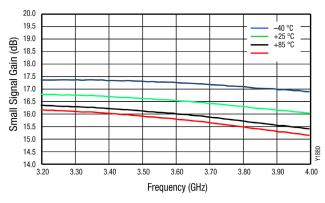
Figure 20. Narrow Band Gain vs Frequency over Temperature
