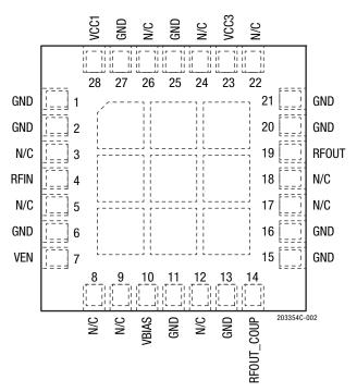
Figure 2. SKY66185-11 Pinout (Top View)
