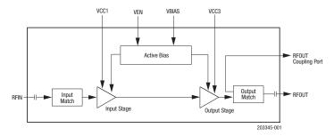
Figure 1. SKY66185-11 Linear PA Block Diagram
