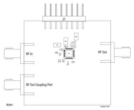
The C3 and C4 components are not required. Some of the other components shown are optional.
