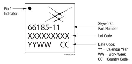
Figure 12. Typical Part Marking
