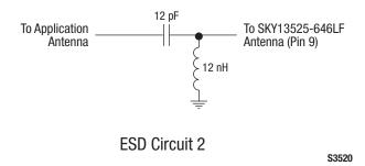
Figure 7. SKY13525-646LF Recommended ESD Protection Circuits
