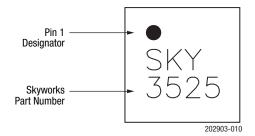
Figure 10. Typical Part Markings (Top View)
