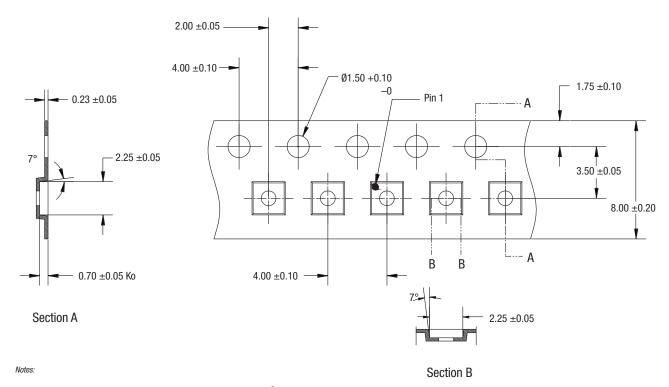
Carrier tape material: black conductive polycarbonate bakeable material at 125  $^\circ$  C Cover tape material: transparent conductive material 5.40 mm width. All measurements are in millimeters.
