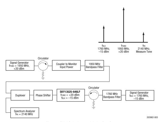
Figure 3. Third Order Intermodulation Test Setup
