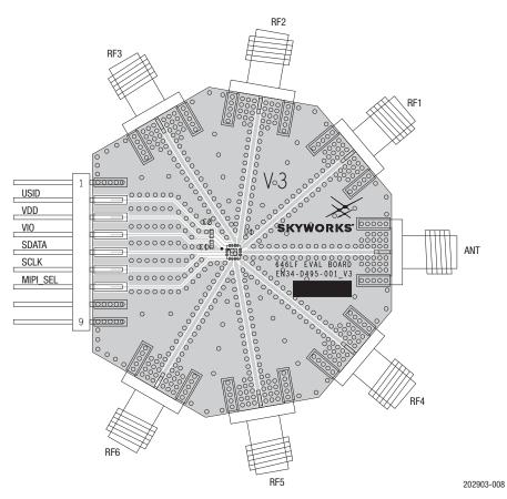
Figure 8. SKY13525-646LF Evaluation Board Assembly Diagram
