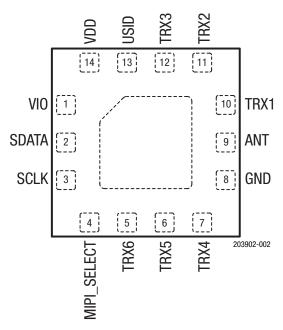
Figure 2. SKY13525-646LF Pinout (Top View)
