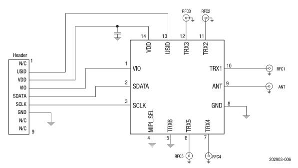
Figure 6. SKY13525-646LF Evaluation Board Schematic
