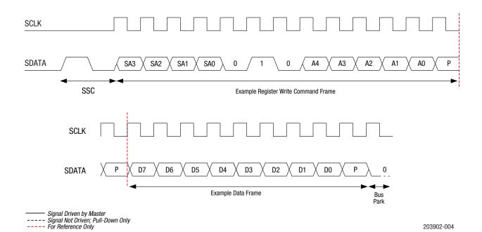
**Figure 4. Register Write Command Timing Diagram**
