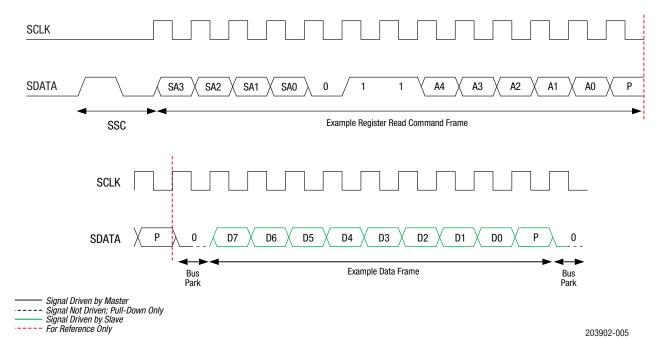
Figure 5. Register Read Command Timing Diagram
