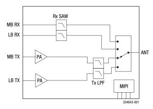
Figure 1. SKY68000-31 Functional Block Diagram
