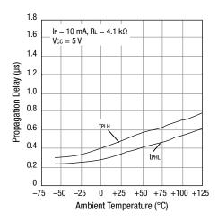
**Figure 4. Propagation Delay vs Temperature**
