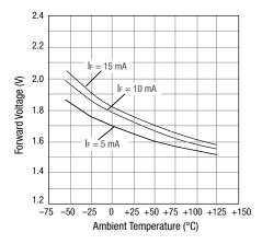
Figure 2. LED Forward Voltage vs Temperature
