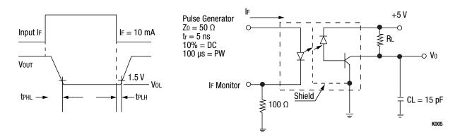
Figure 5. OLH300 Switching Test Circuit
