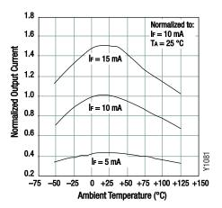
Figure 3. Normalized Output Current vs Temperature
