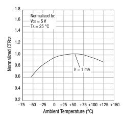
Figure 4. Normalized CTRCE vs Temperature
