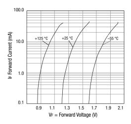
Figure 2. Forward Current vs Diode Forward Voltage
