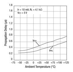
Figure 4. Propagation Delay vs Temperature
