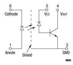
Figure 1. OLI300 Block Diagram
