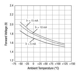
Figure 2. LED Forward Voltage vs Temperature
