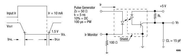
Figure 5. OLI300 Switching Test Circuit
