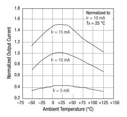
Figure 3. Normalized Output Current vs Temperature
