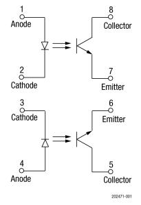
Figure 1. OLS2249 Block Diagram
