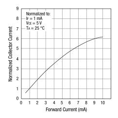
Figure 3. Normalized Collector Current vs Forward Current
