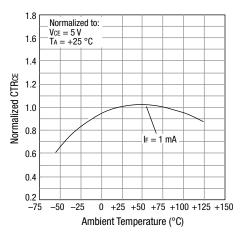
**Figure 4. Normalized CTRCE vs Temperature**
