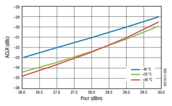
Figure 6. ACLR vs Pout Across Temperature
