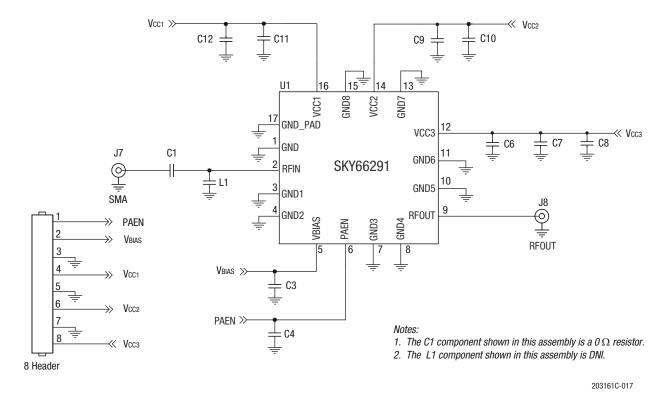
Figure 17. SKY66291-11 Evaluation Board Schematic
