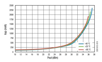
Figure 10. Operating Current vs Pout Across Temperature
