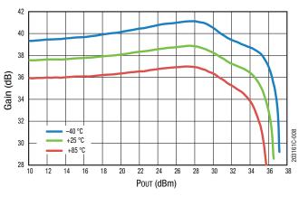
Figure 8. Gain vs Pout Across Temperature
