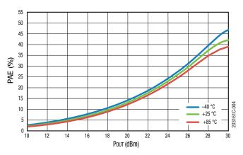
Figure 4. PAE vs. Pout Across Temperature @ 1842.5 MHz, 5 V
