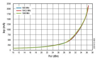
Figure 9. Operating Current vs Pout Across Frequency
