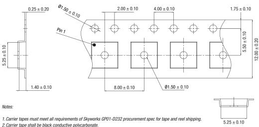
2. Carrier tape shall be black conductive polycarbonate.
