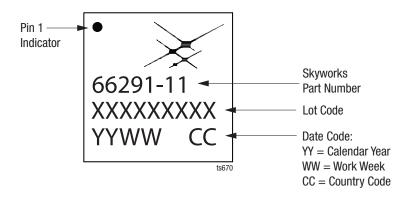
Figure 21. Typical Part Marking for the SKY66291-11
