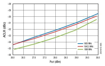
Figure 5. ACLR vs Pout Across Frequency
