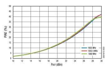
Figure 3. PAE vs Pout Across Frequency @ 5 V, 25 °C
