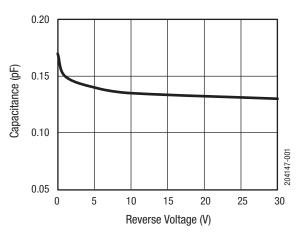
Figure 1. Total Capacitance vs Reverse Voltage
