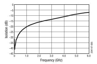
Figure 5. Isolation vs Frequency  $(V_R = 0 V)$
