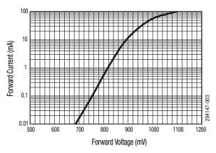
**Figure 3. Forward Current vs Forward Voltage**
