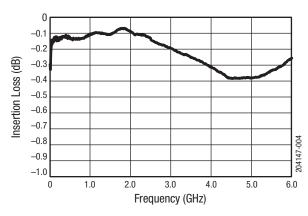
Figure 4. Insertion Loss vs Frequency (IF = 10 mA)
