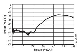
Figure 6. Return Loss vs Frequency (IF = 10 mA)
