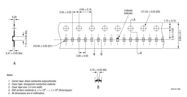
Figure 8. SOD-882 Tape and Reel Drawing
