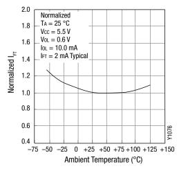
**Figure 3. Normalized Current vs Temperature**
