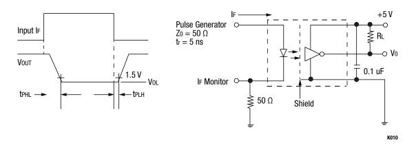
Figure 6. OLF500 Switching Test Circuit
