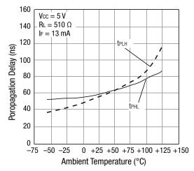
Figure 5. Propagation Delay vs Temperature
