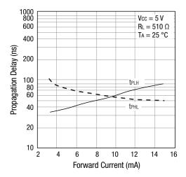
**Figure 4. Propagation Delay vs Input Forward Current**
