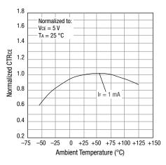
Figure 4. Normalized CTRCE vs Temperature
