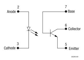
Figure 1. OLH1249 Block Diagram
