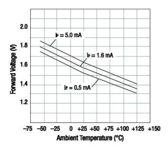
Figure 2. LED Forward Voltage vs Temperature
