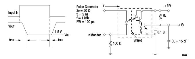
Figure 6. OLH400 Switching Test Circuit
