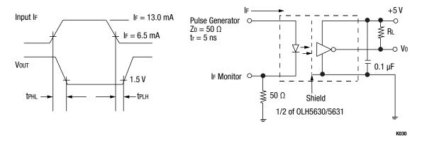
Figure 6. 0LH5630/5631 Switching Test Circuit
