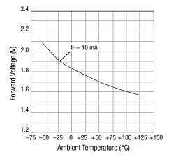
Figure 2. LED Forward Voltage vs Temperature
