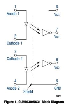
Figure 1 shows the 0LH5630/5631 functional block diagram. Table 1 provides the 0LH5630/5631 absolute maximum ratings.
