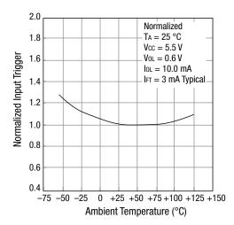
Figure 3. Normalized Input Trigger vs Temperature
