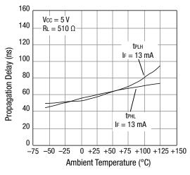
Figure 5. Propagation Delay vs Temperature
