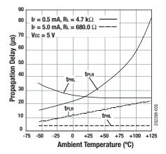
Figure 5. Propagation Delay vs Temperature
