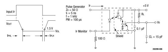
Figure 6. OLH5700/5701 Switching Test Circuit
