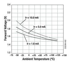
Figure 2. Forward Voltage vs Temperature
