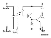
Figure 1. OLH5700/5701 Block Diagram
