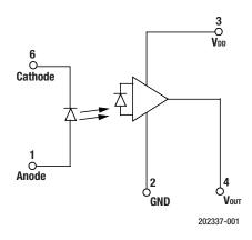
Figure 1. OLI580 Block Diagram
