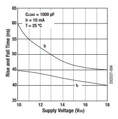
Figure 4. Rise and Fall Time vs Supply Voltage
