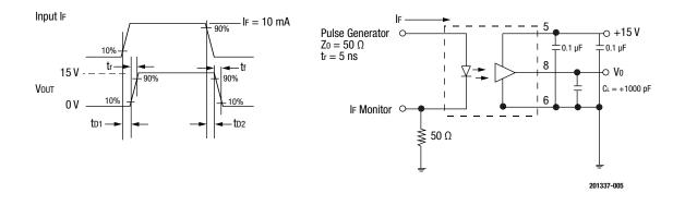
Figure 6. OLI580 Switching Test Circuit
