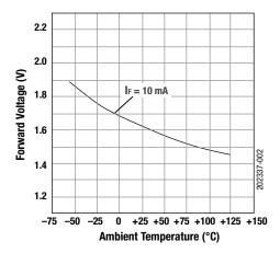
Figure 2. Forward Voltage vs Temperature
