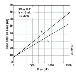
Figure 3. Rise and Fall Time vs Capacitive Load
