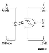
Figure 1. OLI600 Block Diagram
