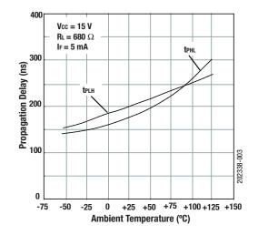
Figure 3. Propagation Delay vs Temperature
