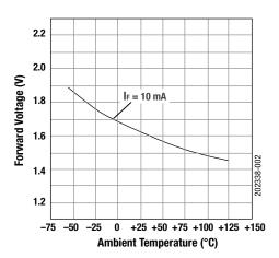
Figure 2. Forward Voltage vs Temperature
