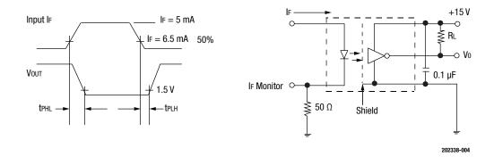
Figure 4. OLI600 Switching Test Circuit
