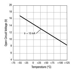
Figure 6: Open Circuit Voltage vs Temperature
