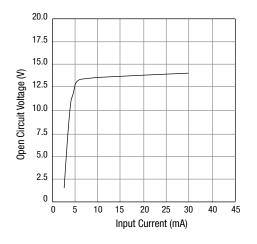
Figure 4. Open Circuit Voltage vs Input Current
