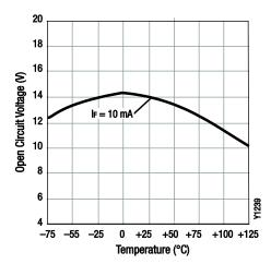
Figure 6: Open Circuit Voltage vs Temperature
