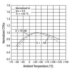
Figure 4. Normalized CTRCE vs Temperature
