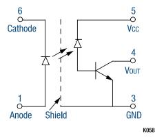
Figure 1. OLS303 Block Diagram
