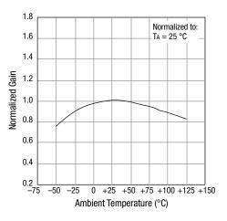
Figure 3. Normalized Gain vs Temperature
