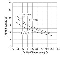
Figure 2. LED Forward Voltage vs Temperature
