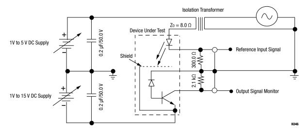
Figure 5. OLS303 Gain and Bandwidth Test Circuit
