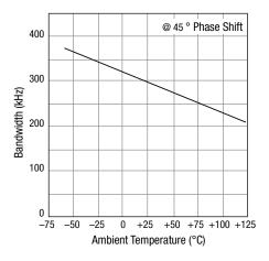
Figure 4. Bandwidth vs Temperature
