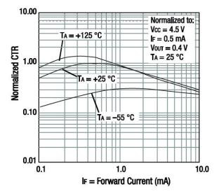
Figure 3. Normalized CTR vs Input Diode Forward Current
