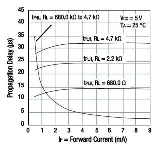
Figure 4. Propagation Delay vs Input Diode Forward Current
