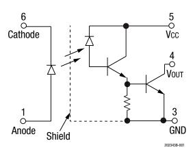
Figure 1. OLS400 Block Diagram
