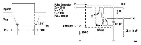
Figure 6. OLS400 Switching Test Circuit
