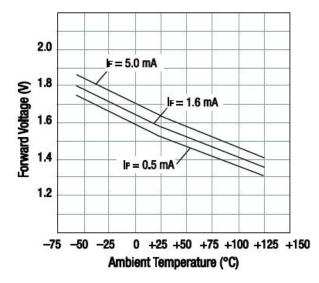
**Figure 2. Forward Current vs Temperature**
