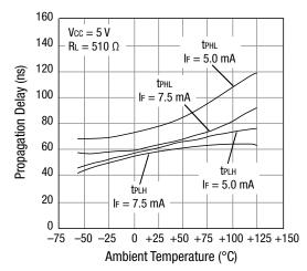
Figure 5. Propagation Delay vs Temperature
