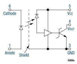
Figure 1. OLS500 Block Diagram
