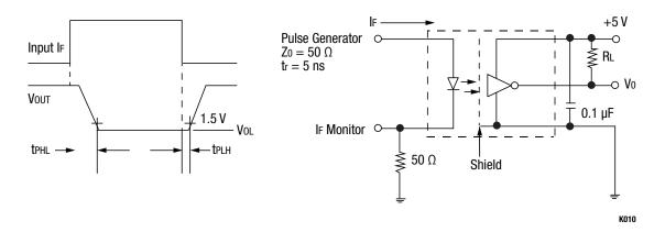
Figure 6. OLS500 Switching Test Circuit
