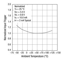
**Figure 3. Normalized Input Trigger Current vs Temperature**
