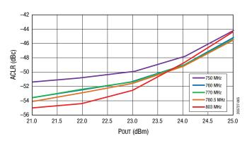
Figure 5. ACLR vs POUT Across Temperature
