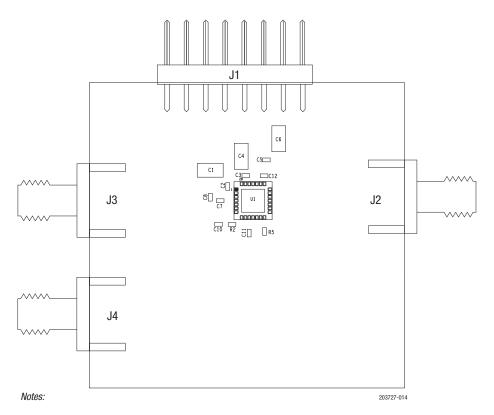
The C3 and C4 components are not required. Some of the other components shown are optional.
