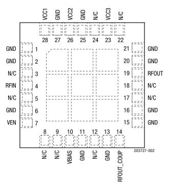
Figure 2. SKY66188-11 Pinout (Top View)
