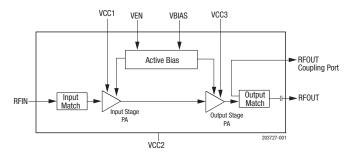
Figure 1. SKY66188-11 Linear PA Block Diagram
