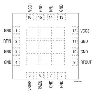
Figure 2. SKY66289-11 Pinout (Top View)
