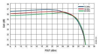
**Figure 19. Gain vs POUT Across Frequency**
