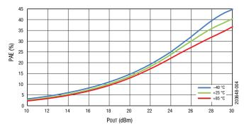
**Figure 3. PAE vs POUT Across Frequency**
