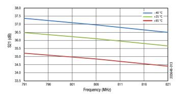
Figure 13. Small Signal Gain vs Frequency Across Temperature
