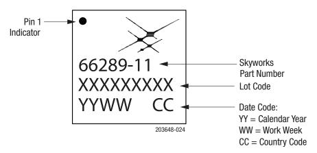
Figure 24. Typical Part Marking
