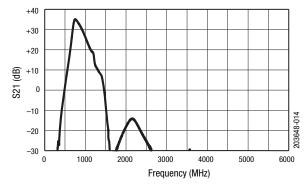
Figure 14. Wide Band Small Signal Gain vs Frequency
