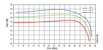
Figure 7. Gain vs POUT Across Frequency
