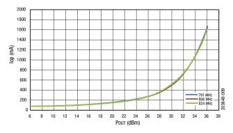
Figure 9. Operating Current vs POUT Across Frequency
