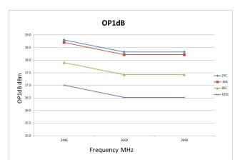
Figure 7. Output 1dB Compression Point
