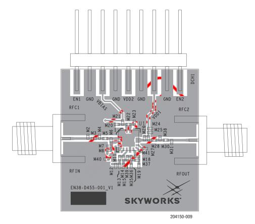
Figure 9. SKY67179-306LF Evaluation Board Assembly Diagram
