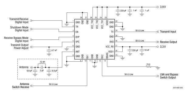
Figure 3. SKY65366-21 Typical Application Schematic
