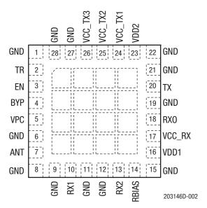
Figure 2. SKY65366-21 Pinout (Top View)
