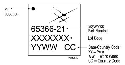
Figure 5. SKY65366-21 Typical Part Marking (Top View)
