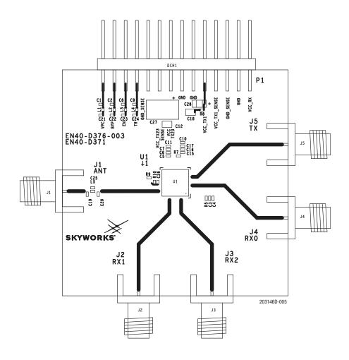
Figure 6. SKY65366-21 Evaluation Board Assembly Diagram
