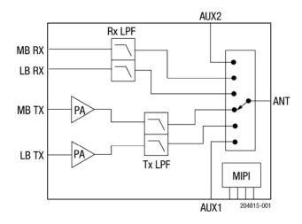
Figure 1. SKY68020-11 Functional Block Diagram
