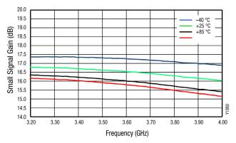
Figure 20. Narrow Band Gain vs Frequency over Temperature
