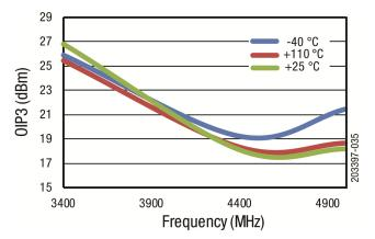
Figure 35. OIP3 vs Frequency over Temperature
