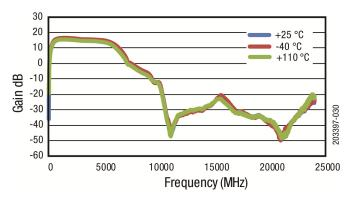
Figure 30. Gain vs Frequency over Temperature
