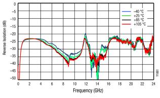
Figure 21. Broadband Reverse Isolation vs Frequency over Temperature
