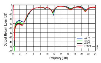
Figure 11. Broadband Output Return Loss vs Frequency over Temperature
