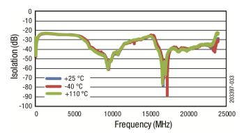
Figure 33. Isolation vs Frequency over Temperature
