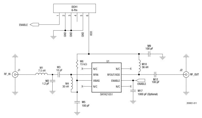
Figure 38. SKYA21051 Evaluation Board Schematic (Optimized for 760 MHz)
