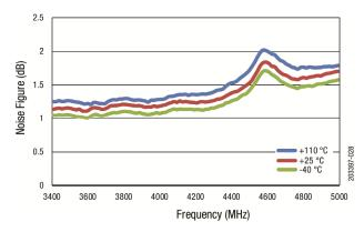
Figure 28. Evaluation Board NF vs Frequency over Temperature
