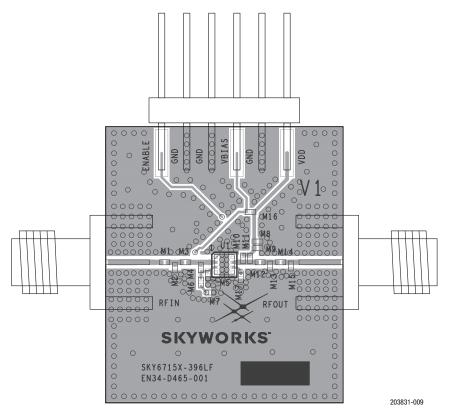
Figure 36. SKYA21051 Evaluation Board Assembly Diagram
