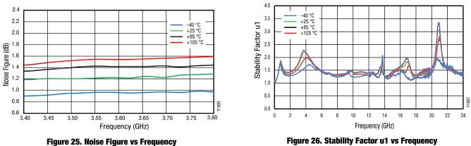
Figure 26. Stability Factor u1 vs Frequency
