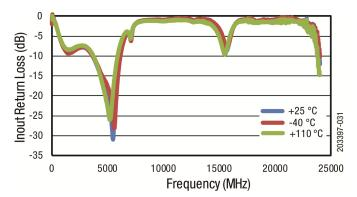
Figure 31. Input Return Loss vs Frequency over Temperature
