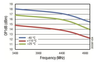
Figure 34. OP1dB vs Frequency over Temperature
