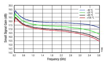
Figure 4. Narrow Band Gain vs Frequency over Temperature
