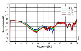
Figure 9. Broadband Reverse Isolation vs Frequency over Temperature
