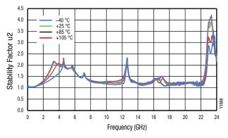
Figure 27. Stability Factor u2 vs Frequency
