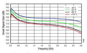
Figure 29. Gain vs Frequency over Temperature
