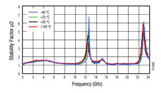
Figure 13. Stability Factor (µ2) vs Frequency over Temperature
