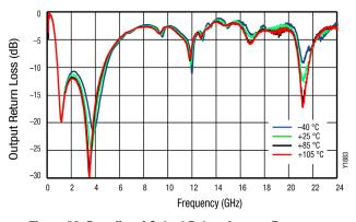
Figure 23. Broadband Output Return Loss vs Frequency over Temperature
