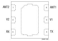
Figure 2. SKYA21070 Pinout (Top View)
