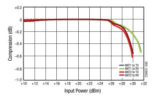
Figure 8. Compression vs Input Power @ 2.50 GHz and 3 V
