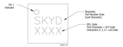
Figure 13. Typical Part Markings (Top View)
