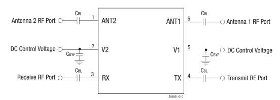
Figure 10. SKYA21070 Evaluation Board Schematic
