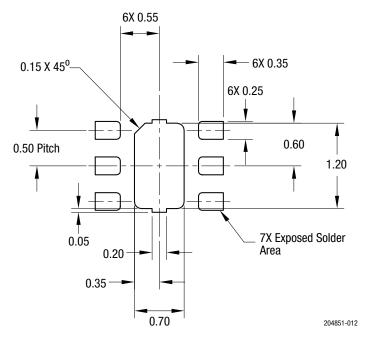
Figure 12. SKYA21070 PCB Layout Footprint (Top View)
